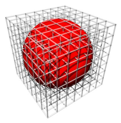
The center is the location for which neighbor objects should be found within a given radius. In this example 68 cells out of 343 do not intersect the query sphere and should ideally not be considered.
