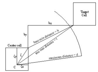
Considering the query center position inside the center cell in multiple dimensions allows to reject cells at maximum distance when  $b \leq d < t$ .
